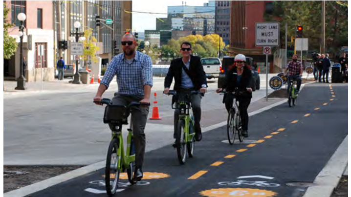
This design focuses on different paving materials and marking types to highlight the bike lane. St Paul, MN
