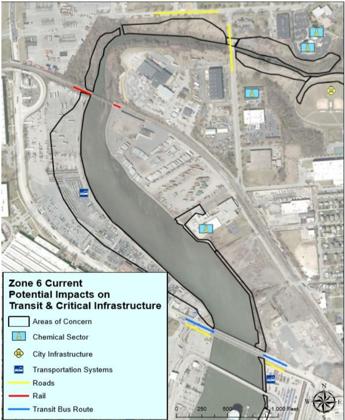
Figure 32: Zone 6 nuisance flooding effects on critical and city-owned infrastructure, along with affected transit routes based on current conditions
