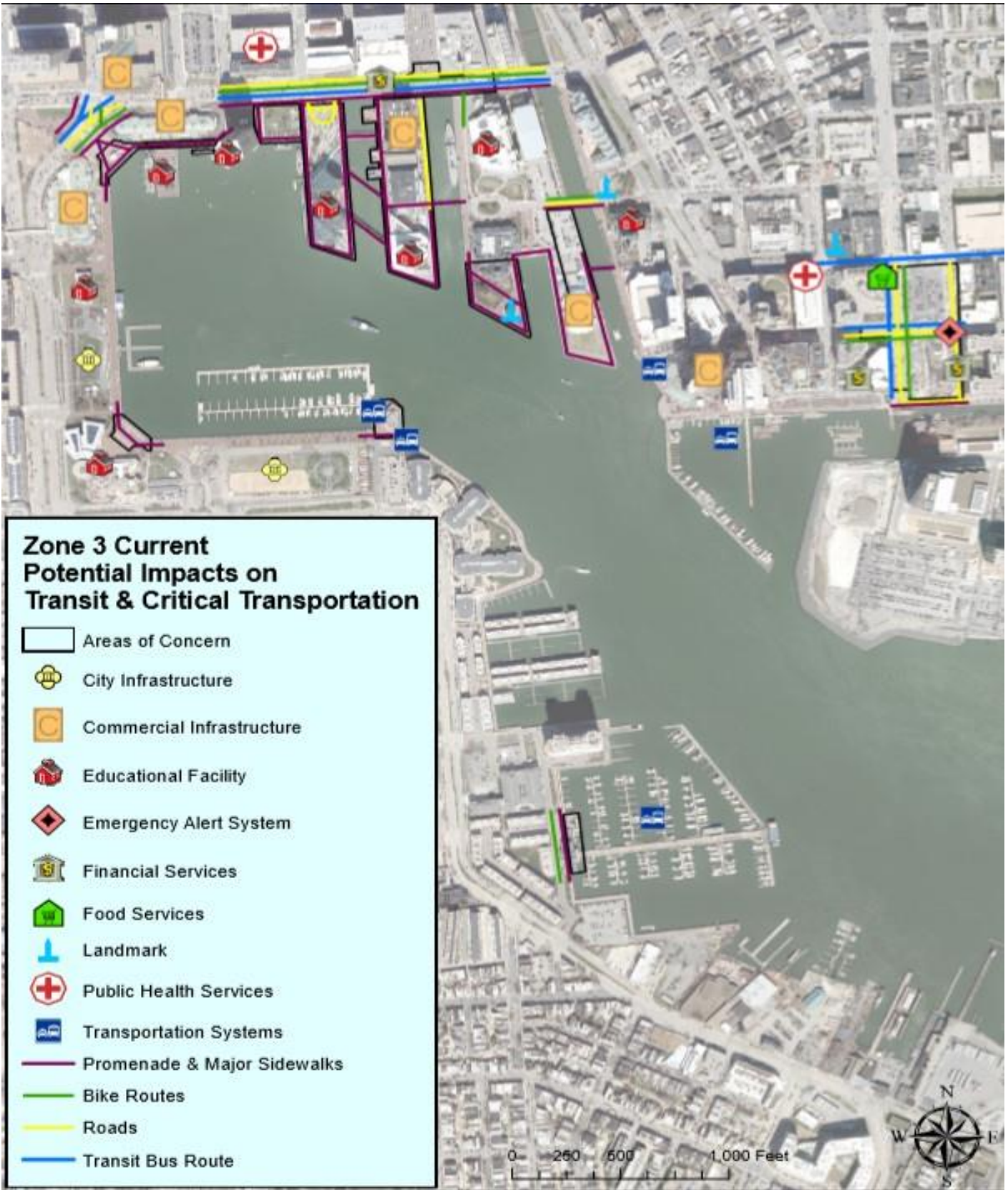
Figure 23: Zone 3 nuisance flooding effects on critical and city-owned infrastructure, along with affected transit routes based on current conditions
